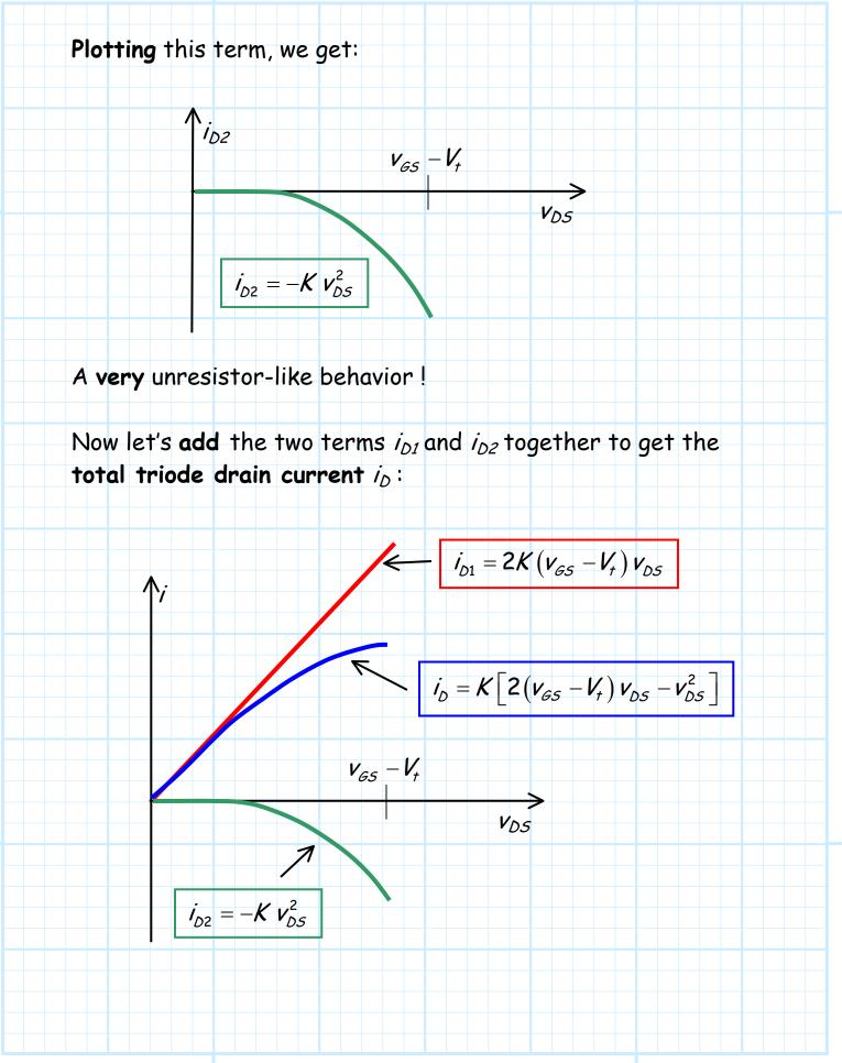
It is apparent that the second term  $i_{D2}$  works to **reduce** the total drain current from its "**resistor-like**" value  $i_{D1}$ . This of course is physically due to the **reduction in channel conductivity** as  $v_{DS}$  increases.
